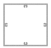
• **Gutter Profile:** In bioclimatic system, aluminum gutter profiles on size of 230 \* 250 \* 3 mm are used for providing water drenage.
